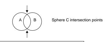
The sphere of satellite C will intersect the area between sphere A and sphere B in only two spots. Your location can be determined by eliminating the location that is within the planet or high into the atmosphere. A  $4^{th}$  satellite signal sphere would only intersect the three other spheres in one location thereby determining the user's precise location.
